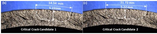
Figure 17. There are no features in either of the areas shown in Blade Figures 68b or 68c that suggest the existence of a fracture origin.
