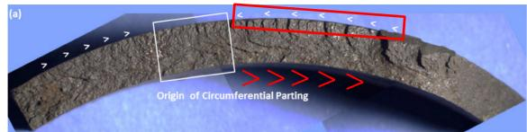
Figure 15. Figure 68 from page 72 of Blade main report. Red rectangle encloses backward chevron marks drawn by Blade. Red chevron marks inserted above are consistent with chevron marks present on the fracture surface. Blade misidentifies the chevron marks as flowing towards the origin. Based on both my physical inspection on February 27-28, 2020, and my analysis of this image, the chevron marks travel to the right, as indicated by the red arrows at the bottom of the figure.
