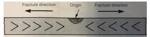
Note the classic chevron or herringbone marks that point toward the origin of the fracture, where there usually is some type of stress concentration, such as a welding defect, fatigue crack, or stress-corrosion crack. The plane of the fracture is always perpendicular to the principal tensile stress that caused the fracture at that location.
