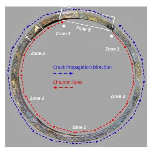
Figure 13. Left: Figure 69 from Blade main report. Right: Corrected Figure 69 showing actual crack growth direction.
